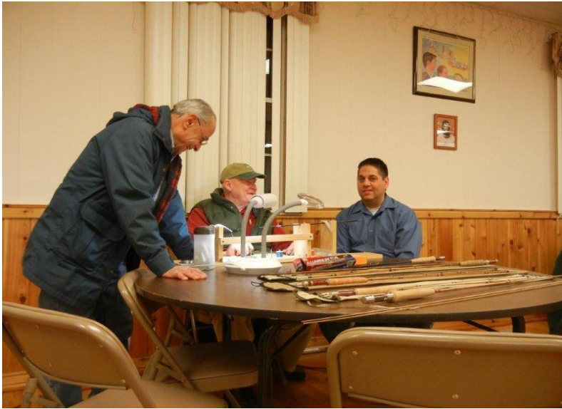
Bob Walsh demonstrates how to wrap a guide on a graphite blank.
